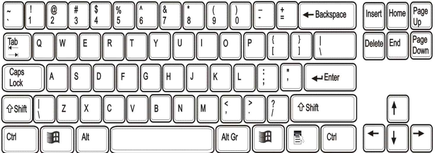
International traditional keyboard (note new “International key” next to left Shift key)
